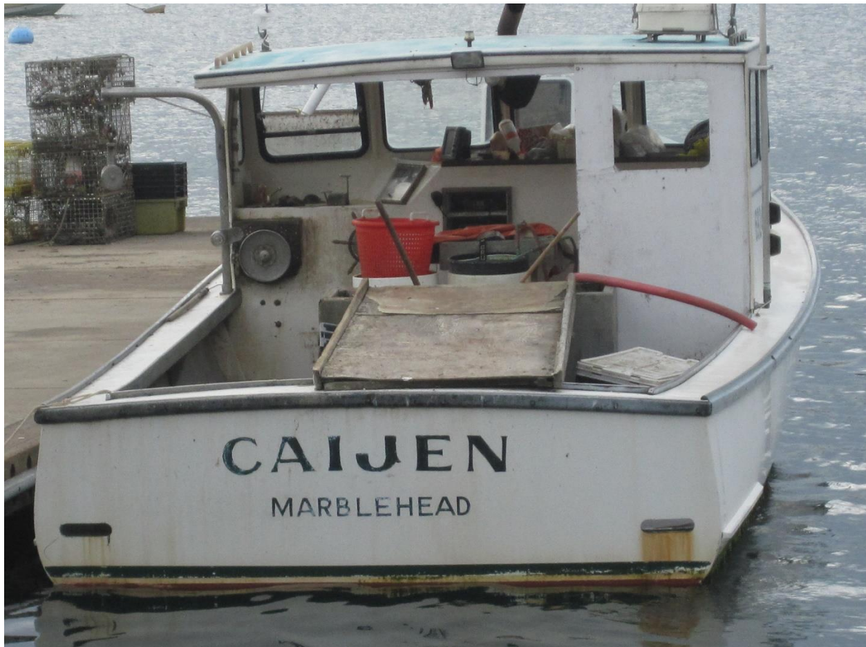
Lobster boat model showing davit and open winch (just to the right of the steering wheel) used for hauling traps.
